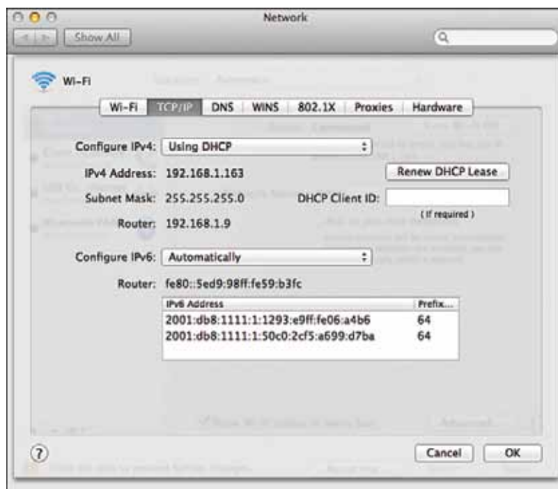
Figure 28-11 Three IPv6 Settings for Dynamic Address Assignment on Mac OS
