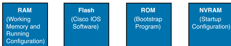
Figure 7-9 Cisco Switch Memory Types
