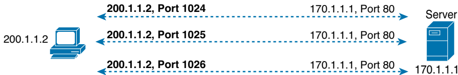
Figure 24-7 Three TCP Connections from One PC
