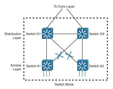
Figure 17-1 A Typical Redundant Network Design
