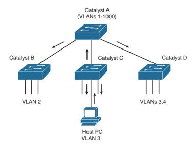
Figure 5-4 Flooding in a Catalyst Switch Network
