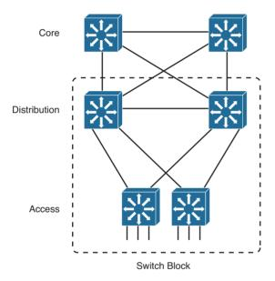
Figure 1-9 Fully Redundant Hierarchical Network Design
