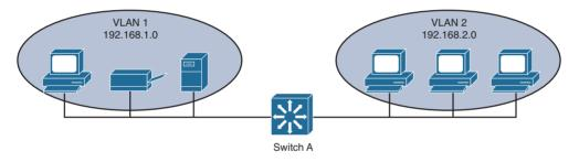
**Figure 1-2** Example of Network Segmentation
