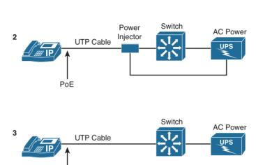
Figure 3-1 Methods to Supply Power to a Networked Device
