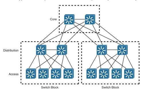
Figure 1-16 A Redundant Core Layer
