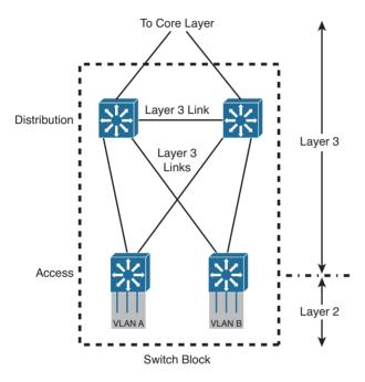
Figure 1-15 A Completely Routed Switch Block
