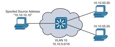
**Figure 21-1** *Using a Spoofed Address Within a Subnet*
