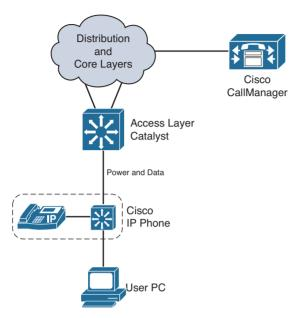
Figure 4-6 Basic Connections to a Cisco IP Phone
