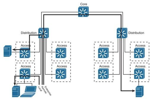
**Figure 1-7** *Traffic Flow Paths Through a Network Hierarchy*
