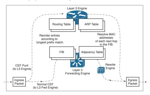
Figure 11-3 Packet Flow Through a CEF-Based Multilayer Switch
