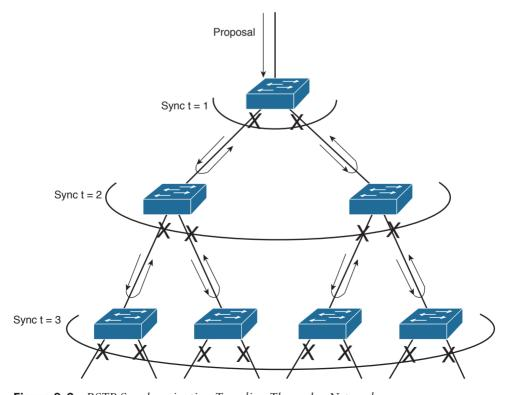
**Figure 9-2** RSTP Synchronization Traveling Through a Network
