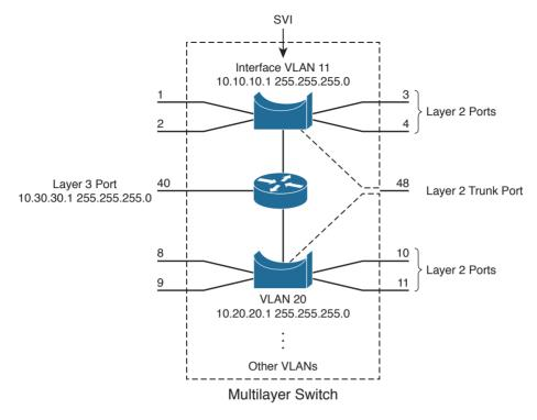
**Figure 11-2** Catalyst Switch with Various Types of Ports
