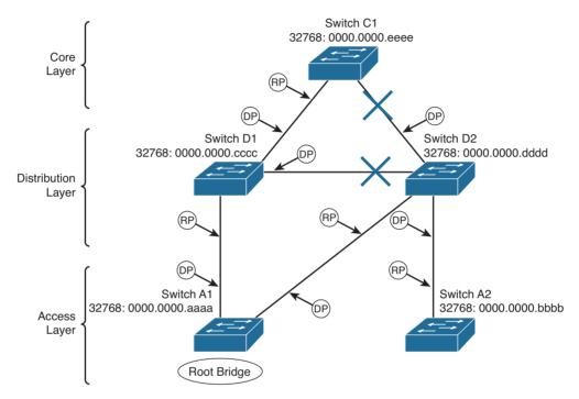
Figure 7-2 Campus Network with STP Converged
