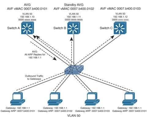
**Figure 18-3** *Multilayer Switches in a GLBP Group*
