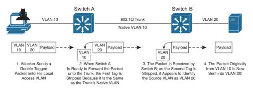
Figure 20-3 VLAN Hopping Attack Process
