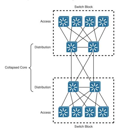
Figure 1-18 A Collapsed Core Network Design
