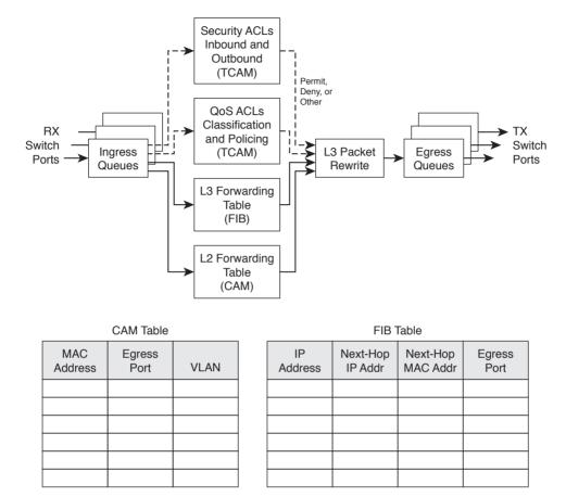
Figure 2-4 Operations Within a Multilayer Catalyst Switch
