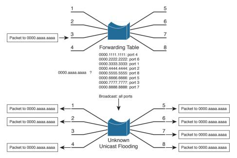
Figure 2-2 Unknown Unicast Flooding
