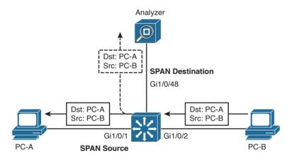
**Figure 16-2** *Using Local SPAN to Monitor Transmitted Traffic*
