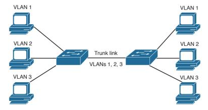
Figure 4-3 Passing VLAN Traffic Using Single Links Versus a Trunk Link
