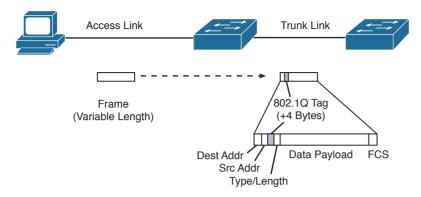
Figure 4-5 IEEE 802.1Q Frame-Tagging Standard
