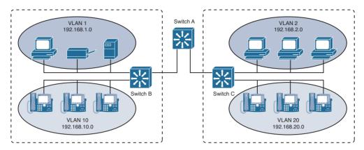
Figure 1-4 Network Growth Through New VLANs
