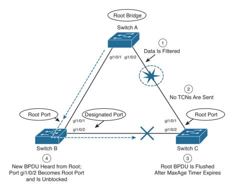
Figure 6-8 Effects of an Indirect Topology Change
