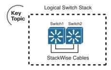
**Figure 17-6** *Creating a Logical Switch with StackWise*
