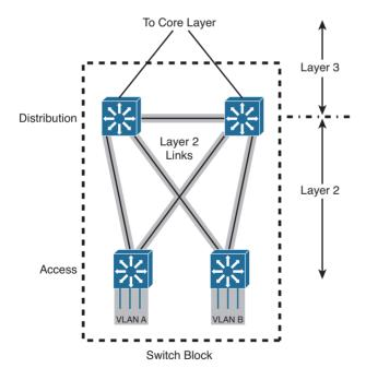
**Figure 1-13** A Redundant Switch Block Design
