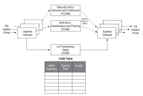
**Figure 2-3** Operations Within a Layer 2 Catalyst Switch
