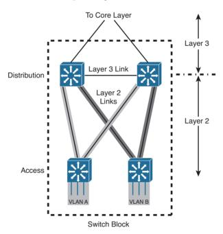
**Figure 1-14** Best Practice Loop-Free Switch Block Topology
