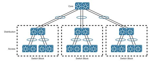
Figure 17-5 Enhanced Logical Switched Network Architecture
