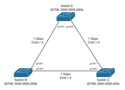
**Figure 6-3** Example of Root Bridge Election
