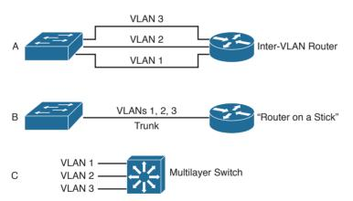
**Figure 11-1** Examples of Inter-VLAN Routing Connections
