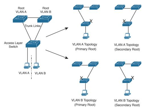
**Figure 9-3** Possible STP Topologies for Two VLANs
