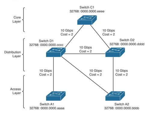
Figure 7-1 Campus Network with an Inefficient Root Bridge Election
