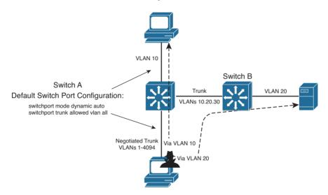
Figure 20-2 An Example of Switch Spoofing to Gain Access to a Trunk
