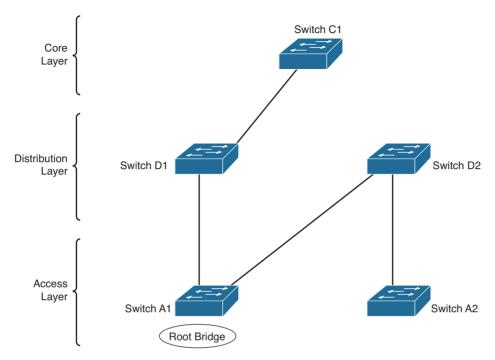
**Figure 7-3** Final Spanning-Tree Structure for the Campus Network
