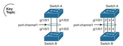
Figure 10-2 Scaling Bandwidth by Bundling Physical Links into an EtherChannel
