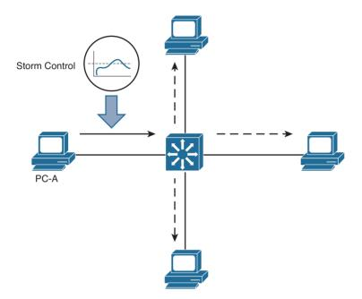
Figure 19-1 Using Storm Control to Limit Received Frames Before They Are Flooded
