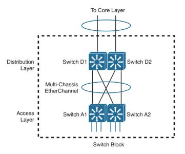
Figure 17-3 Connecting Two Logical Switches with an EtherChannel
