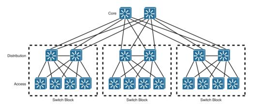
Figure 1-12 Network Growth by Adding New Switch Blocks
