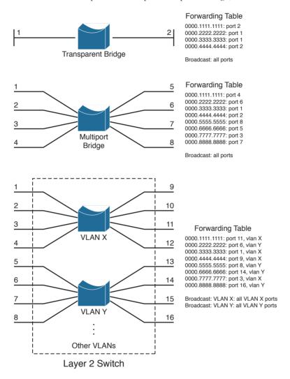
**Figure 2-1** A Comparison of Transparent Bridges and Switches
