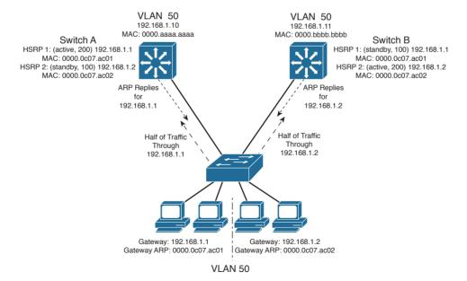
**Figure 18-2** Load Balancing with Two HSRP Groups
