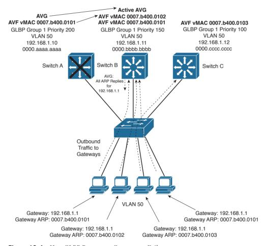
**Figure 18-4** How GLBP Reacts to a Component Failure
