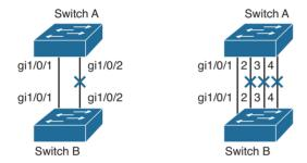
Figure 10-1 The Effects of Trying to Scale Bandwidth with Individual Links
