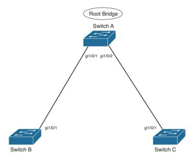
**Figure 6-6** *The Resulting STP Topology*
