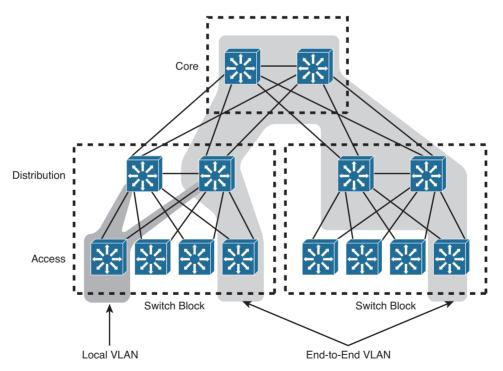
Figure 4-2 The Extent of an End-to-End VLAN
