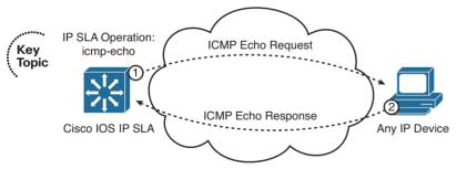
Figure 15-1 IP SLA ICMP Echo Test Operation
