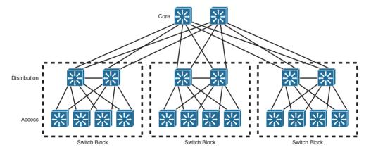
Figure 17-4 Traditional Redundant Switched Network Architecture
