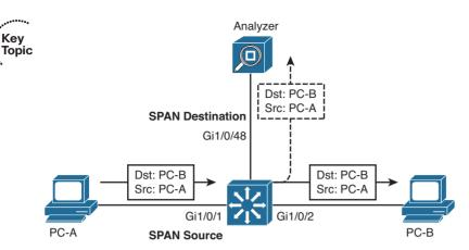
Figure 16-1 Using Local SPAN to Monitor Received Traffic
