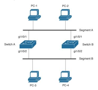
**Figure 6-2** *Redundant Bridging with Two Switches*
