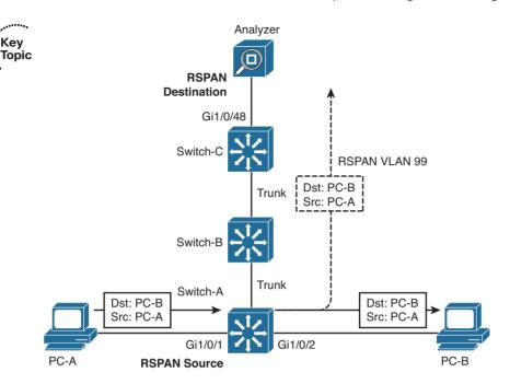
Figure 16-3 Using RSPAN to Mirror Traffic Across Multiple Switches
