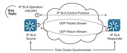
Figure 15-2 IP SLA UDP Jitter Test Operation
