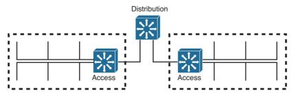
Figure 1-5 Two-Layer Network Hierarchy Emerges
