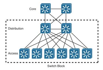
Figure 1-11 Network Growth by Adding Access Switches to a Switch Block
