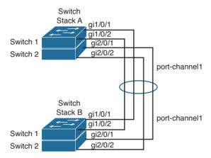
Figure 10-3 Increasing Availability with a Multichassis EtherChannel
