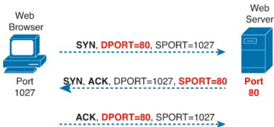
Figure 5-5. TCP Connection Establishment
