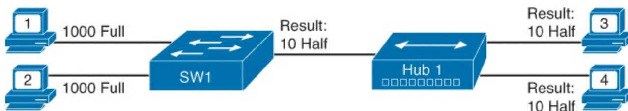
Figure 6-15. IEEE Autonegotiation with a LAN Hub
