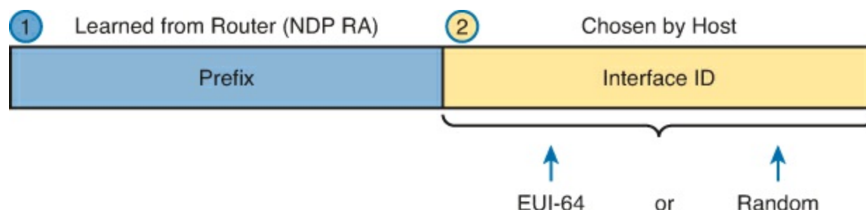
Figure 28-9. Host IPv6 Address Formation Using SLAAC
