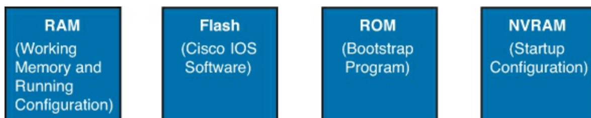
Figure 7-9. Cisco Switch Memory Types
