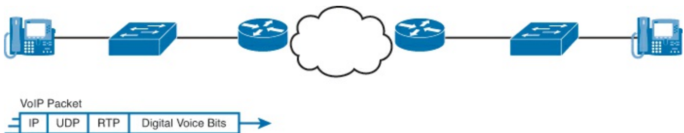
Figure 5-8. IP Packet Sent by a Voice Call
