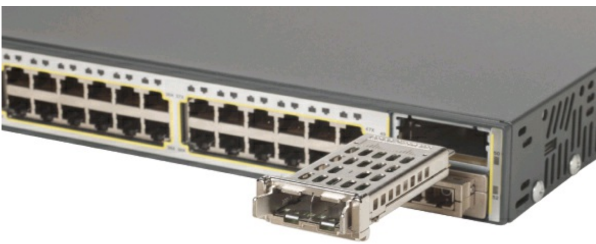
Figure 2-8. Gigabit Fiber SFP Sitting Just Outside a Switch SFP Port
