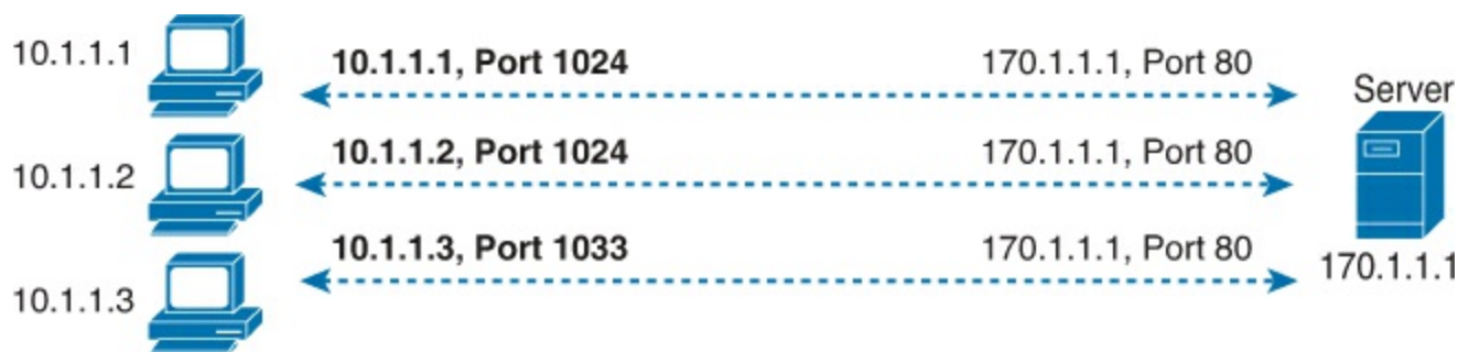
Figure 24-6. Three TCP Connections from Three PCs
