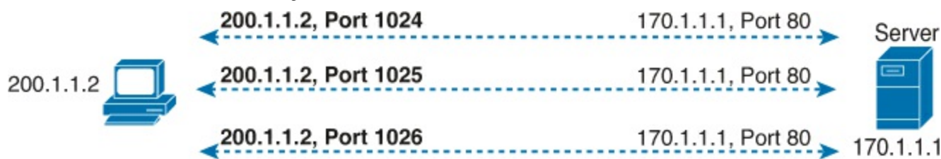
Figure 24-7. Three TCP Connections from One PC
